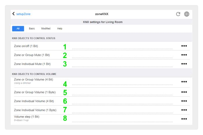
1 - enter a KNX group address (GA) here to switch the zone on or off by a 1-bit message with value 1 or 0. switching on means to play the most recent selected source again.
