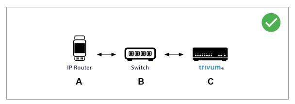
Multicast basically means: device (A) (IP router) gives a KNX message "1/2/3 1bit 1" to the network switch (B), and tells that switch to send this to all other devices in the network.
